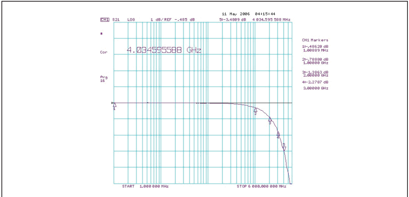
Fig 5: Typical Insertion Loss Plot from 1MHz to 6.0GHz, Vcc=1.8V, 25C
